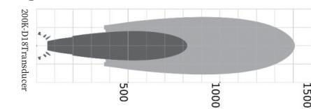
Dark color: 25mm diameter PVC pipe Unit: mm
