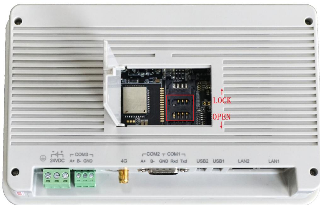
Figure 25 HMI installation of 4G card
