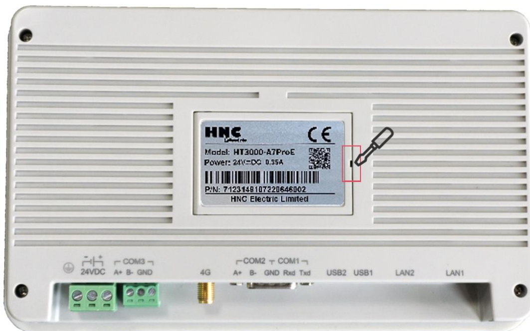
Figure 24 HMI 4G card backplane
