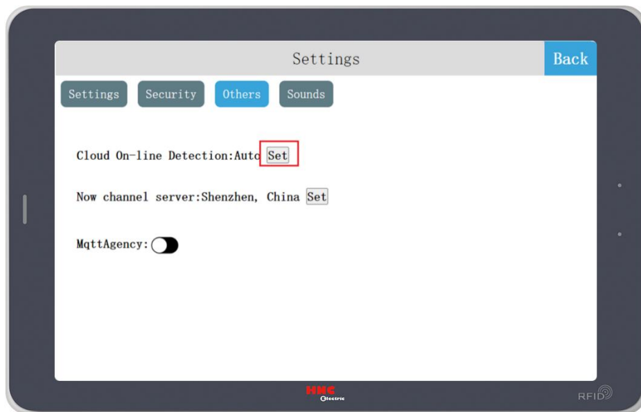
Figure 48 Setting Cloud Online Detection Frequency
