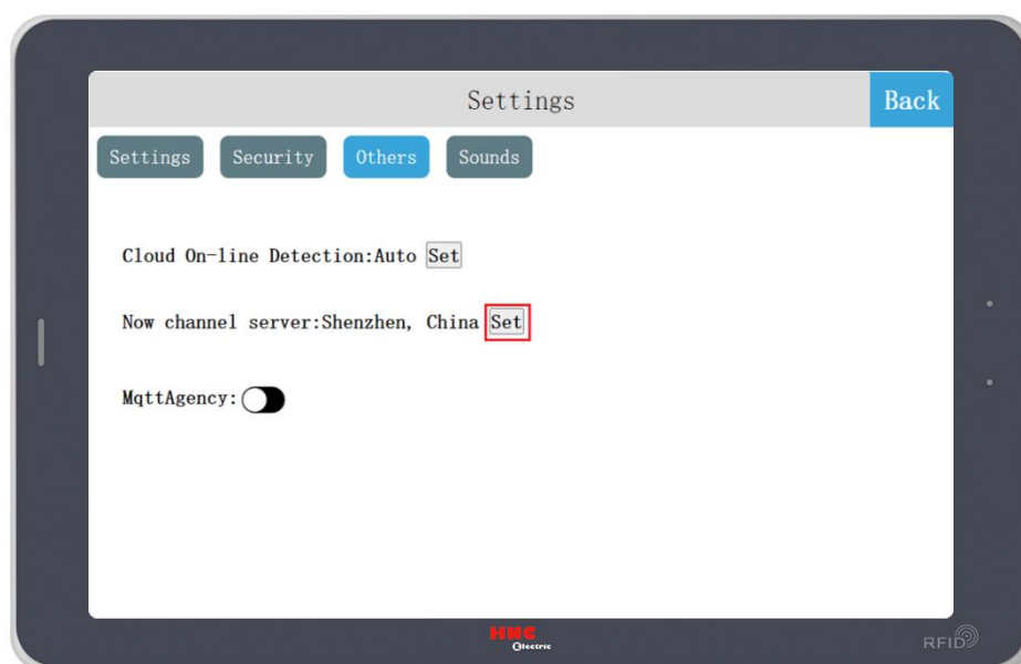
Figure 50: Setting the Current Channel Server
