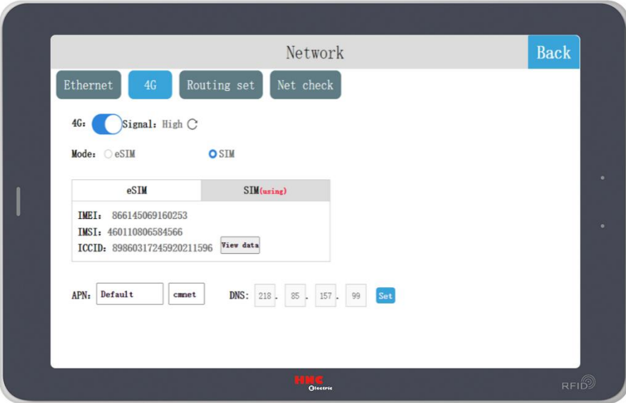
Figure 85 Enabling the SIM card
