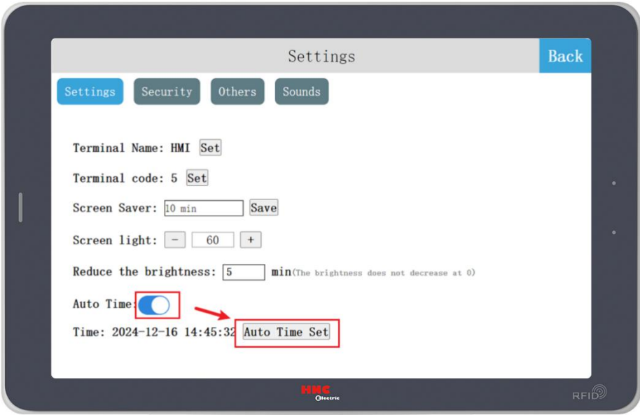
Figure 33 Setting Network Timing 1
