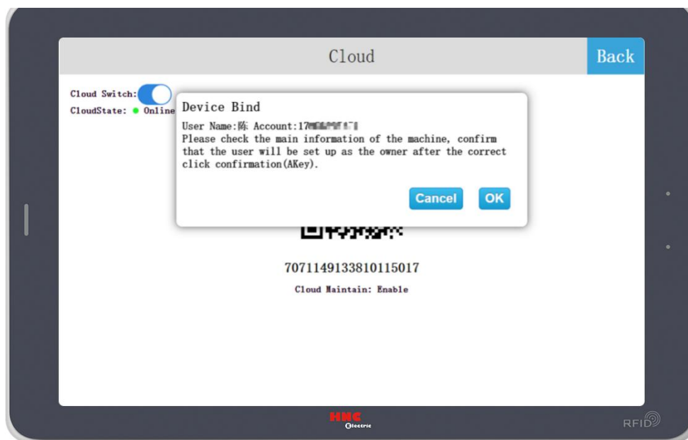
Figure 70: Determination of binding for HMI cloud settings
